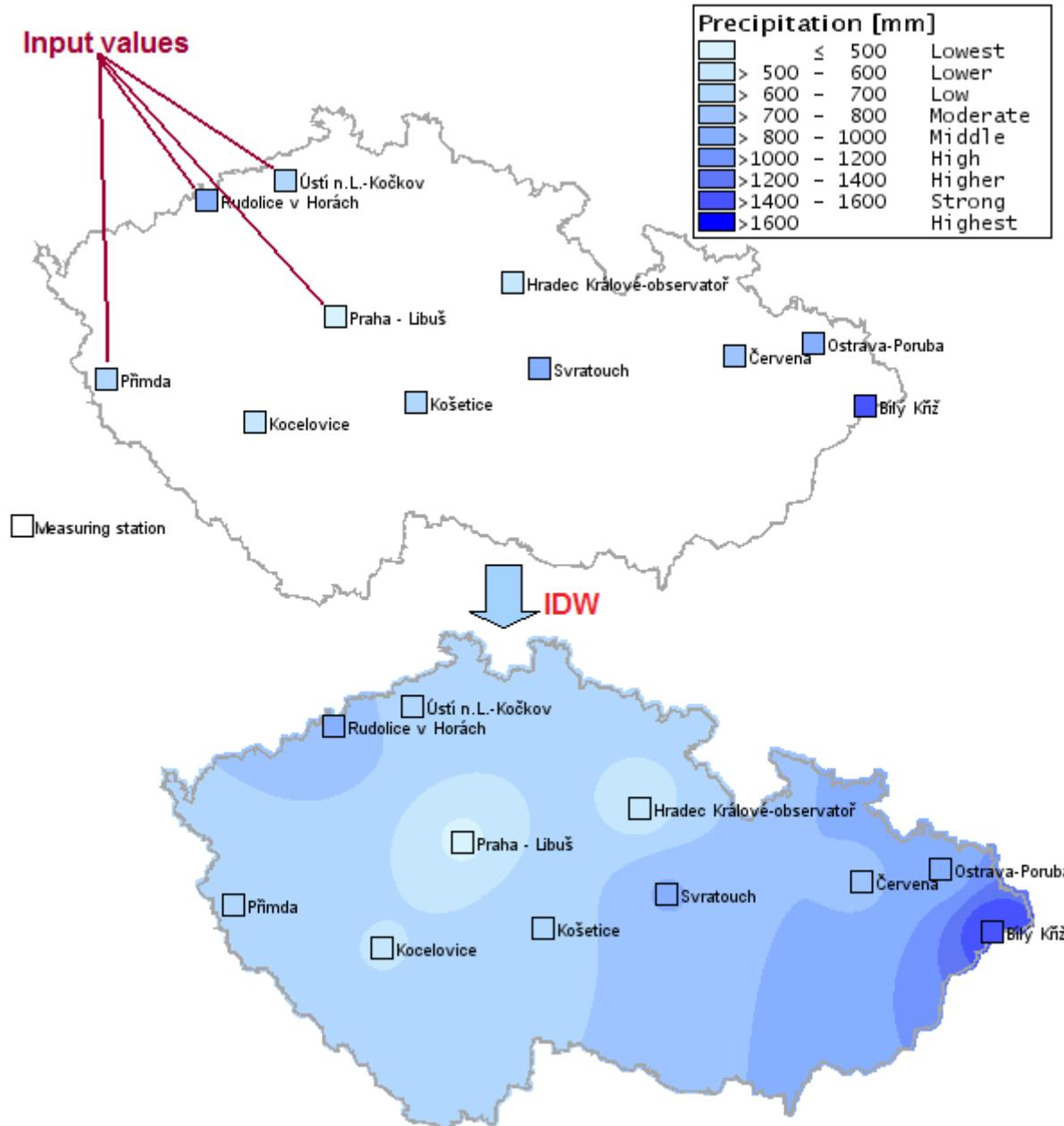
**IDWInterpolator** computes for each cell in computed matrix its value, and those values can be converted to colors using color scale and used for drawing map background.
