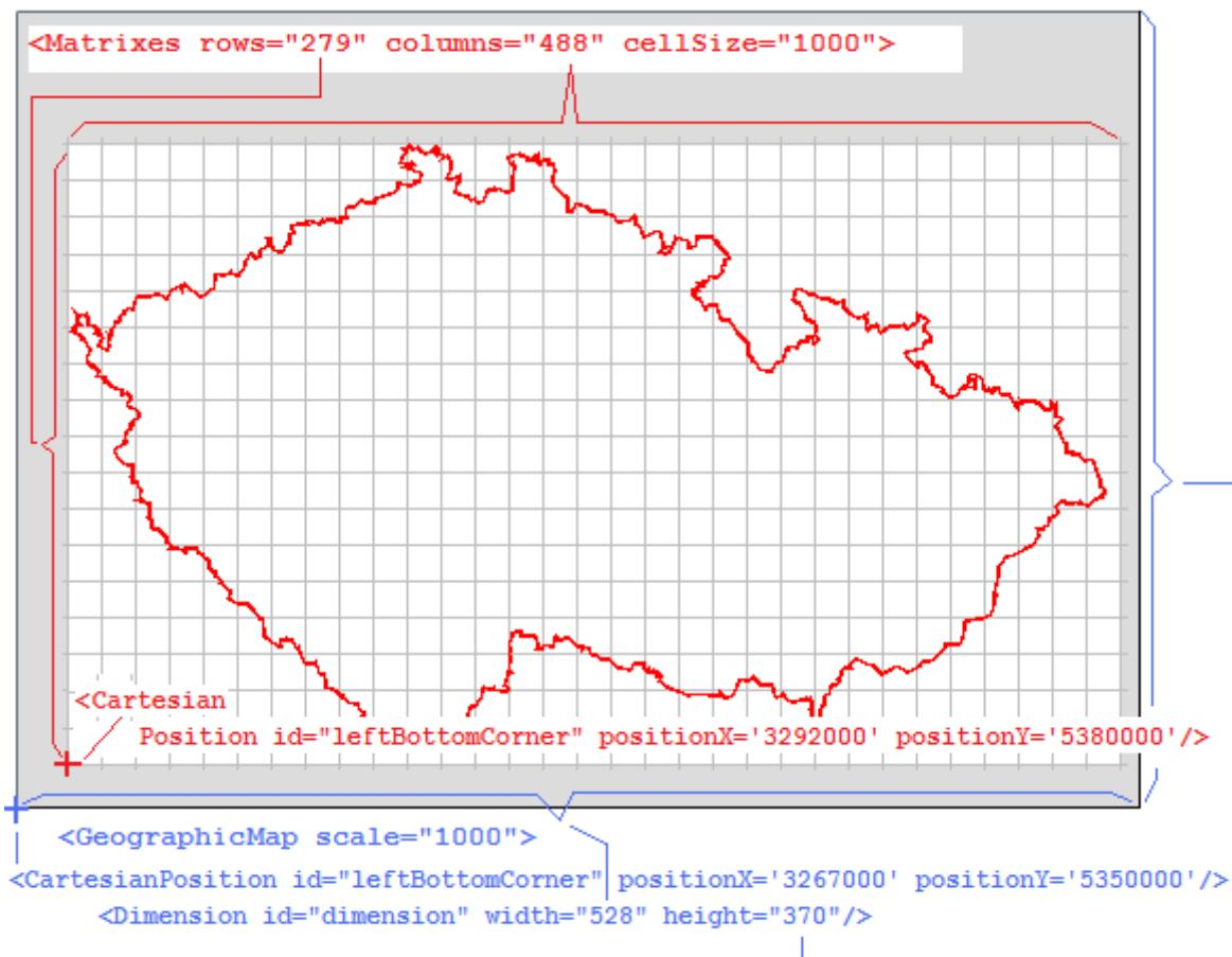
On this map, there is 25 pixels void space on left side:  $(3292000 / 1000) - (3267000 / 1000) = 25\text{px}$ , and 61 pixels on top:  $(370 - 279) - ((5380000 / 1000) - (5350000 / 1000)) = 61$
