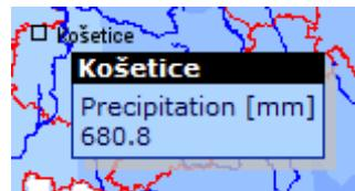
Tooltip contain information about name of the place where input value are obtained and it value. Background color is given from color scale.
